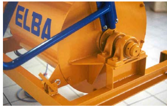
Maintenance-free bearing. Slewing security device via mechanical pin.
