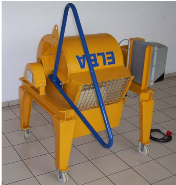
EMS 60 in discharge position with removed dust cover.
